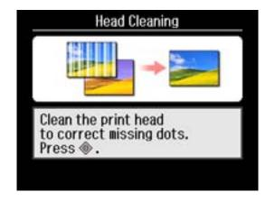
7. Press the ♦ start button to clean the print head. You see a message on the LCD screen during the cleaning cycle.
